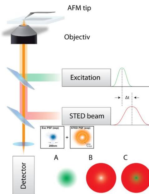
**Fig. 1:** Scheme of an AFM and STED based system showing the major components. The sketch includes the time shifted pulses of the excitation source and the STED beam, the detector unit and the AFM. Schematic of the intensities of excitation laser (A), donut shaped STED laser (B) and the overlapping of both (C). A donut shaped STED beam is most common and it used to provide a lateral resolution enhancement, but it is not the only implementation.
