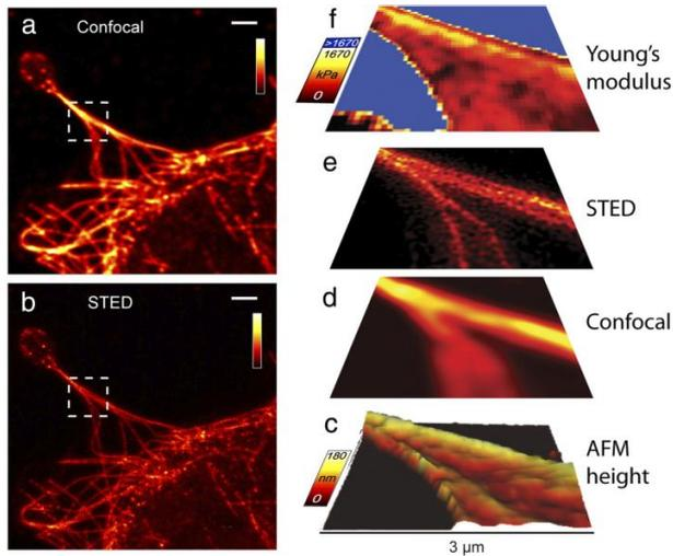
**Fig. 4:** Confocal image (a) and STED image (b) (both raw data) of Atto 647 N labeled microtubules in COS7 cells in PBS. From AFM mapping extracted 3D height image (c) and calculated elasticity map (f) correlated with the STED (e) and confocal image (d) (both linear deconvolved) collected from same area. Scale bars in (a) and (b): 2 μm, axes bars in (c)-(f): 3 μm.
