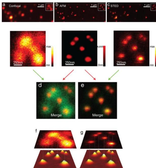
**Fig. 3:** Raw data of confocal (a), AFM (b) and STED measurement (c) of 40nm fluorescent spheres. Zoomed areas of optical images and new AFM scan are highlighted. Overlay of AFM image with the confocal (d) and STED data (e). 3D AFM topography correlated with confocal (f) and STED data (g).
