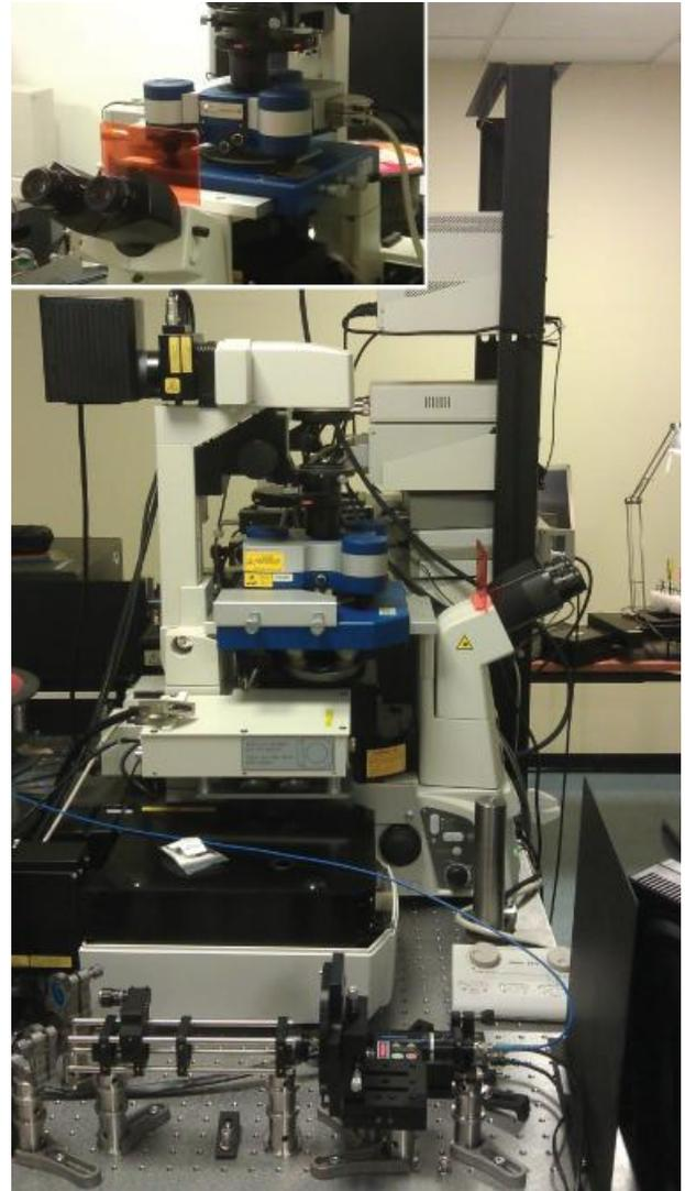
**Fig. 2:** Combined NanoWizard® 3 AFM and Nikon based STED system in the laboratory of Prof. Alberto Diaspro from IIT in Genua, Italy.
