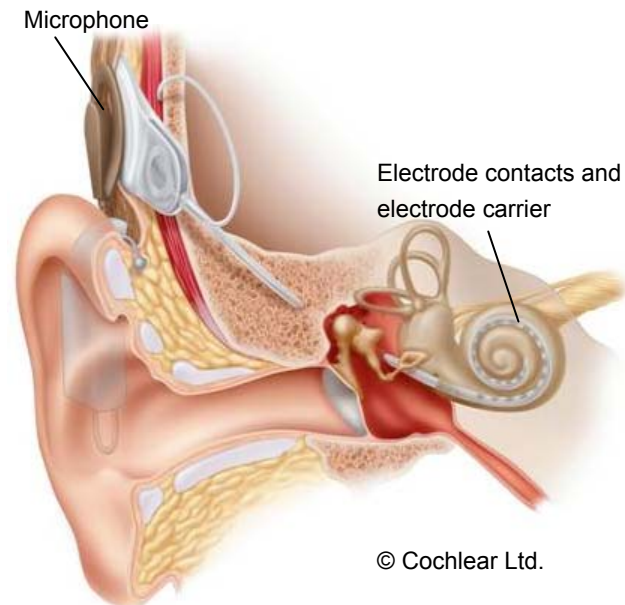
Fig. 1: Components of a Cochlea Implant and their position inside and outside the ear.
